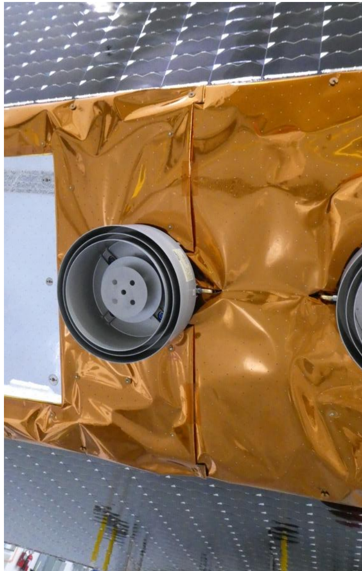
Figure 4-14 GNSS-POD redundant antenna
