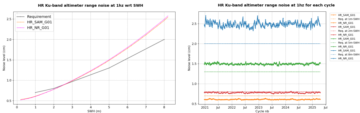
Figure 175: 1 Hz noise of HR Ku-band altimeter range, in cm. Left panel: noise function of SWH in m for Sentinel-6 MF HR and Jason-3; the purple line represents the requirement thresholds. Right panel : noise level computed for each cycle and at 1, 2, 5 and 8 m-wave (solid lines) and the corresponding requirement levels (dashed lines).
