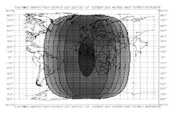
Figure 11 – MSG Level 1.5 ground resolution map (E-W direction)
