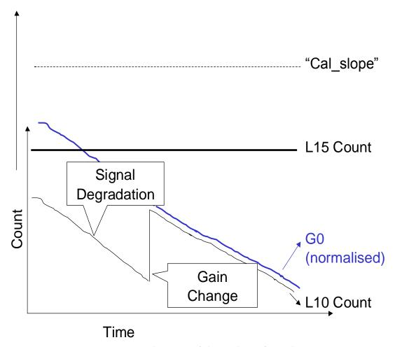
Figure 5 – Schematic of the scaling of Level 1.5 counts
