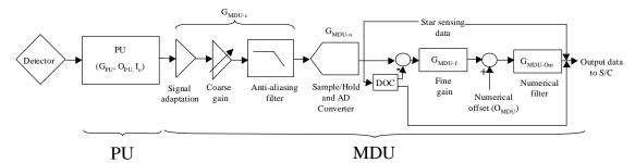
Figure 3 – SEVIRI detection chain
