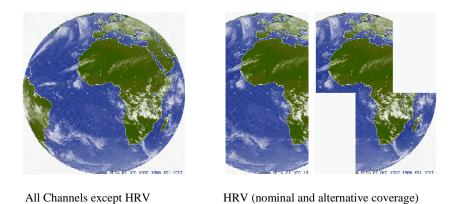
Figure 6 – Nominal Earth coverage of MSG image channels
