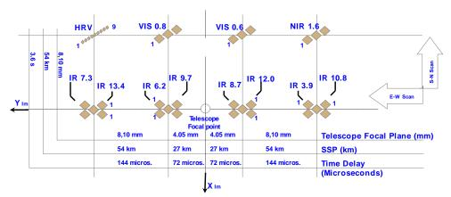
Figure 2 – SEVIRI focal plane arrangement
